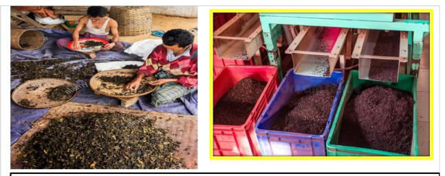
**Sifting or Sorting:** The sorting is done on a roller. Pieces of tough stalk and fibre are removed. The dust and leaves are separated into grades of various shapes and sizes, depending on how they will be sold.
