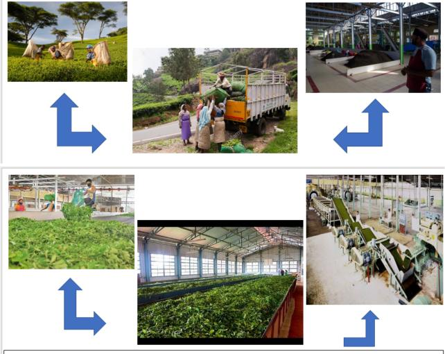
Withering: Tea leaves are gently and evenly laid out on a mesh in out trough. Air is passed through the leaves to dry them. This process removes about 80% of the surface moisture..
